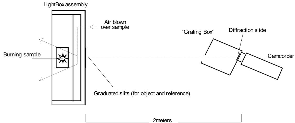
The above diagram illustrates the main components of the setup as seen from above.
